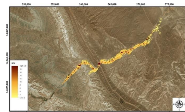
Figure 18. Maximum velocity map for minimum roughness in the piping scenario of Chahchaheh Dam
