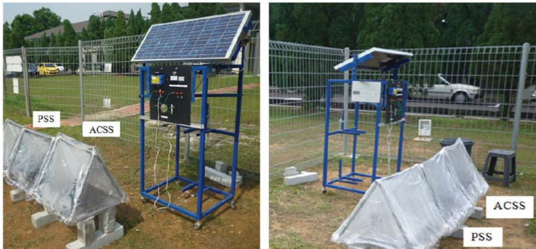
Figure 7. Photograph of experimental setup of ACSS and PSS (Riahi et al., 2019)
