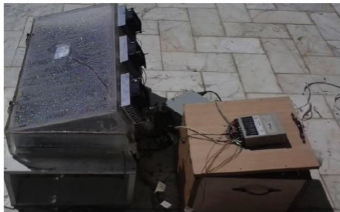
Figure 22. Photograph of the portable asymmetrical solar still (Rahbar et al., 2016).
